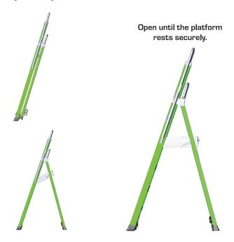
Open the Safety Cage<sup>®</sup> from the side by separating the front and rear rails. As the rails move apart, the platform and will begin to lower. Open until the platform rests securely on the horizontal support on the rear half.
