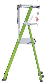
Set Gates to In-Use Position: Press in buttons and raise gates until they lock into place before entering the platform. Make sure gates are securely locked and lower the midspan bar into position before entering the platform.
