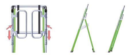
**To Return to Storage Position:** Stand at the front of the Safety Cage<sup>®</sup> and press in the push buttons to lower the gates to their stored position. Close the Safety Cage by pushing up on the platform and bringing the front and rear rails together.
